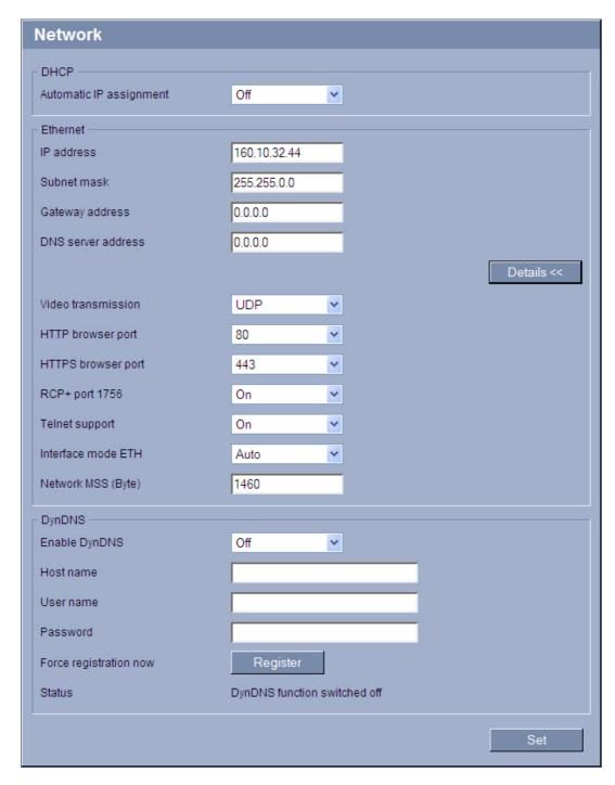
The settings on this page are used to integrate the VIP XD into an existing network. Some changes only take effect after the unit is rebooted. In this case, the **Set** button changes to Set and Reboot.
