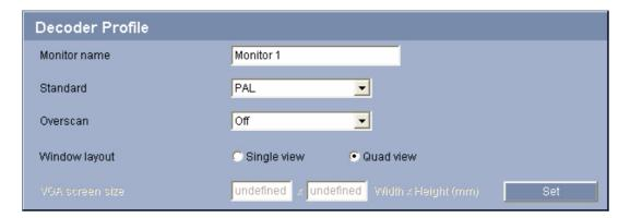
In this screen you can set the various options for the display of video images on an analog monitor or VGA monitor. A number of presets are available for configuring the VGA video output signal. These presets can be adapted to individual requirements if necessary.
