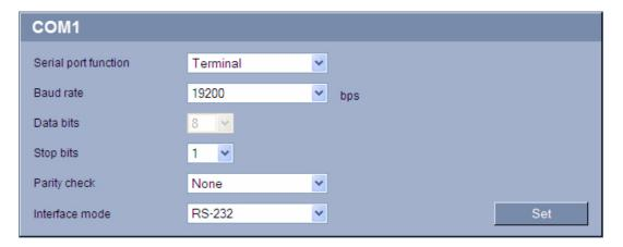
You can configure the serial interface parameters (orange terminal block) to meet your requirements.
