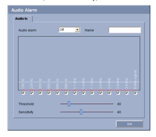
The VIP XD can create alarms on the basis of audio signals. You can configure signal strengths and frequency ranges in such a way that false alarms, for example due to machine noise or background noise, are avoided.
