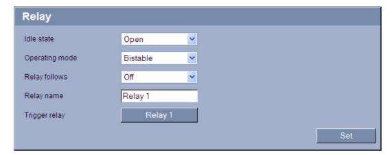
You can configure the switching behavior of the relay output. You can specify an open switch relay (normally closed contact) or a closed switch relay (normally open contact).
