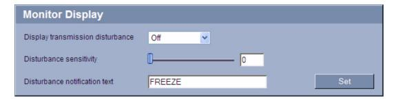
The VIP XD can recognize transmission interruptions and display a warning on the monitor if set accordingly.
