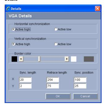
The **Details** window allows you to adapt the video output signal to specific requirements with greater detail. You can also set the frame color for the image border.
