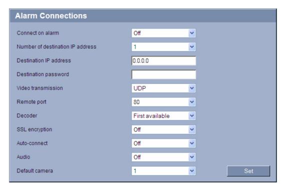
You can select how the VIP XD responds to an alarm. In the event of an alarm, the unit can automatically connect to a pre-defined IP address. You can enter up to ten IP addresses to which the VIP XD will connect in sequence in the event of an alarm, until a connection is made.
